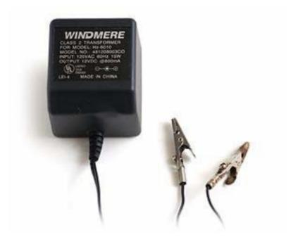
We also recommend that if you are building a bigger unit to use often, that you should get a high end power supply like the Radio Shack Micronta regulated 12V power supply. Do not use more than 3 amps. Most of these come 2.5 amps, which is great.
