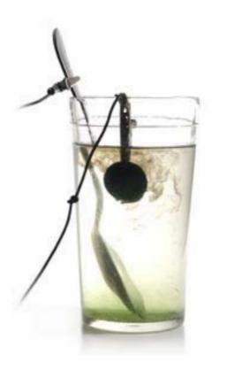
The electrical current is passing through the coin and separating all nonmetallic particles from the coin.
